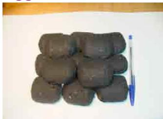
After carbonisation, an agglomeration of these charcoal fines is necessary to facilitate the combustion and transport of the briquettes obtained. The agglomeration techniques are in two main families: compression techniques and pelletisation (a non-compressing technique). The fabrication of briquettes or charcoal nuts demands a binder to mix with the charcoal fines. This binder can either be starch, Arabic gum, molasses or clay.
